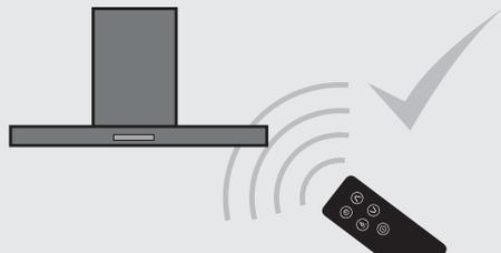
**UNPAIR:** Once in setting mode, press both, the Timer (⌚) and the Light (💡) icons. The led display will show (A) blinking waiting hob's signal. Finally, press the timer icon and the light icon at the same time again to delete all communications over induction hob and remote control.
